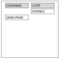
This is to activate the audio output from DOLBY AC3 5.1 DOWNMIX to 2 channel mode. Select the preferred SPEAKER
